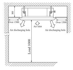
**Space installation needed (unit: mm)**
